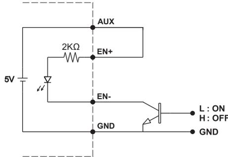
(B) ON / OFF Control by NPN transistor
