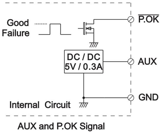
\*Place an additional capacitor to have a better performance of auxiliary power operation.
