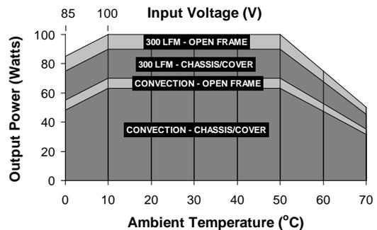
**Derating requirements** – Chart above applies to models 1003 thru 1008 only. 100 Watts 300 LFM forced air, open frame. 70 Watts convection cooled open frame. Derate 10% with chassis and cover. Derate 1.0  $W_{out} / 1 V_{in}$  below 100  $V_{in}$  and between 100  $V_{in}$  and 85  $V_{in}$ . Use larger of the two deratings when using chassis/cover below 100  $V_{in}$ . Derate output power linearly to 50% between 50° and 70° C
